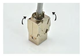
5. Terminate by pushing to close the 2 wings from both sides.
