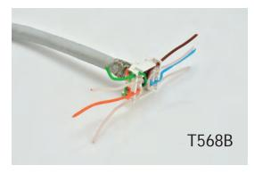
2. Remove the foil from each pair. Seat the wires into the cap according to the wire scheme.
